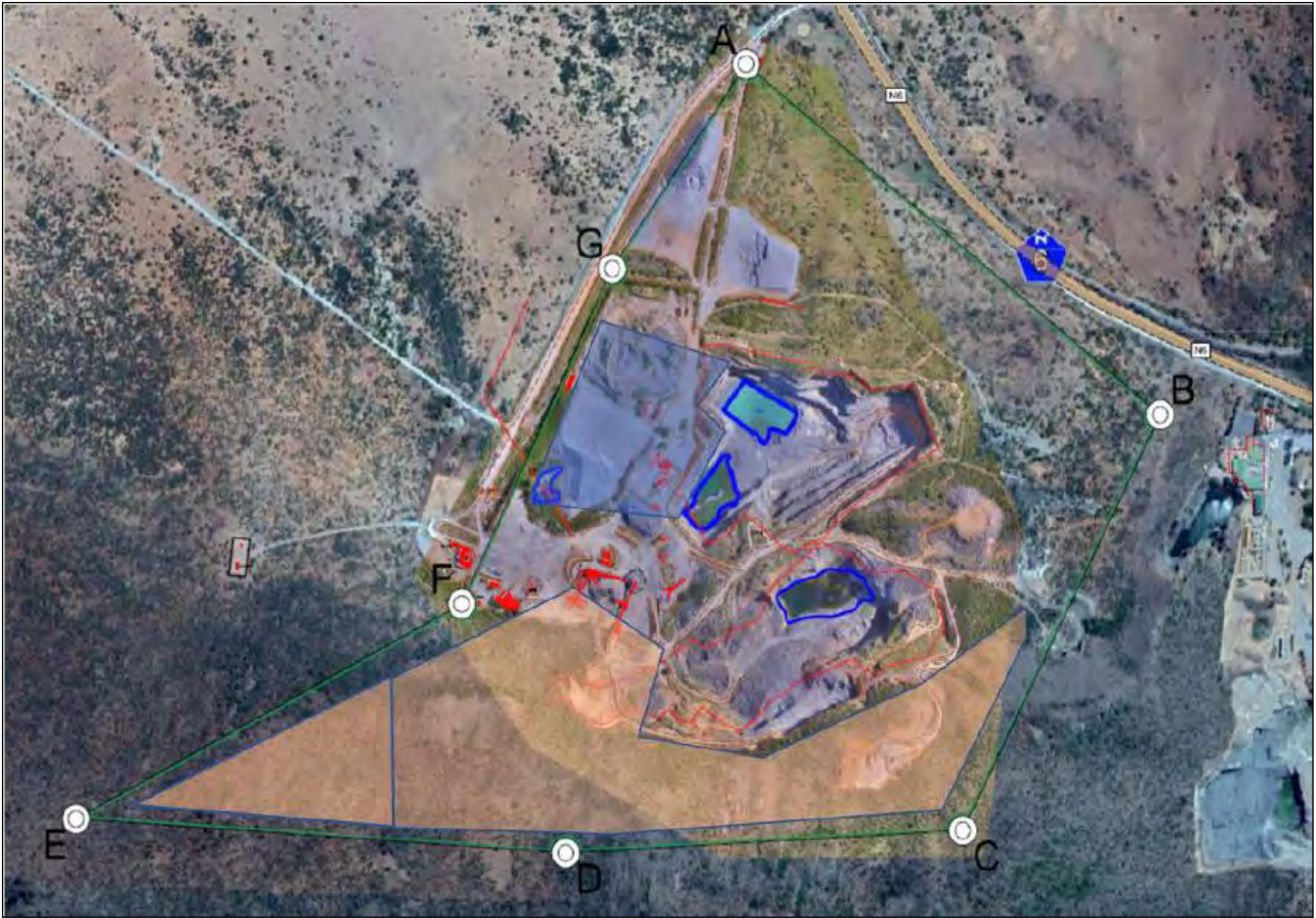
Figure 3: Indication of the future resource to be mined by extending the existing dolerite pit south and west.
