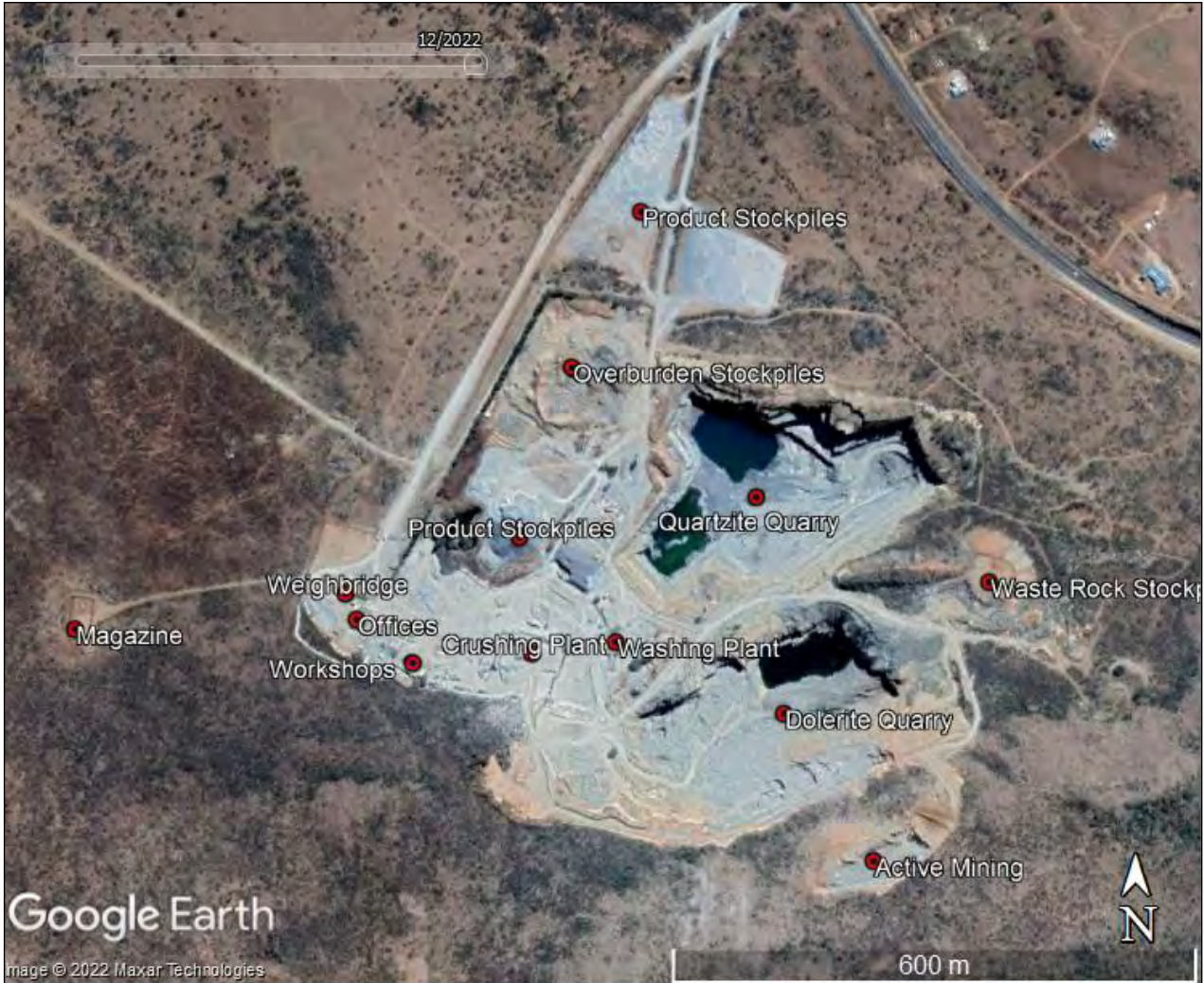
Figure 2: Site layout of Queenstown Quarry indicating the current activities that will continue.
