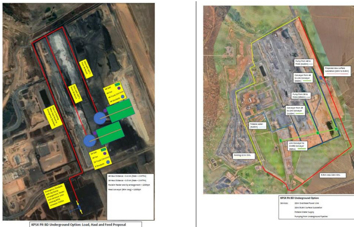
Figure 2-4: Layout for KPSX UG haul roads, pipelines, conveyor, load-haul and feed infrastructure
