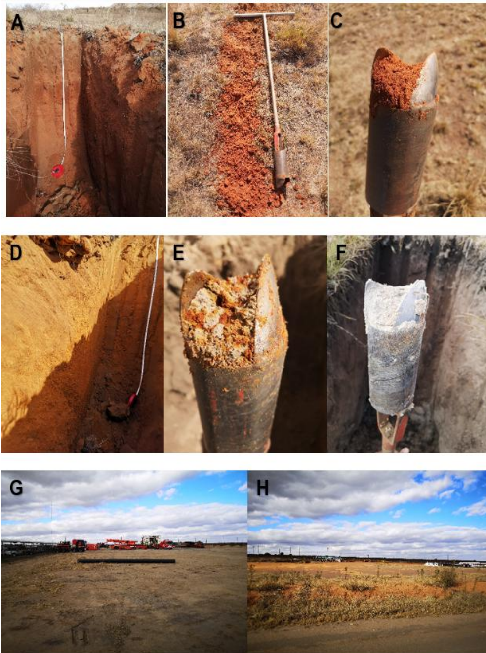
Figure 5-12: Examples of the identified soil forms: A – C) Hutton (Red apedal), D) Clovelly, E) Longlands, F) Albic & G – H) Witbank (Transported Technosols).
