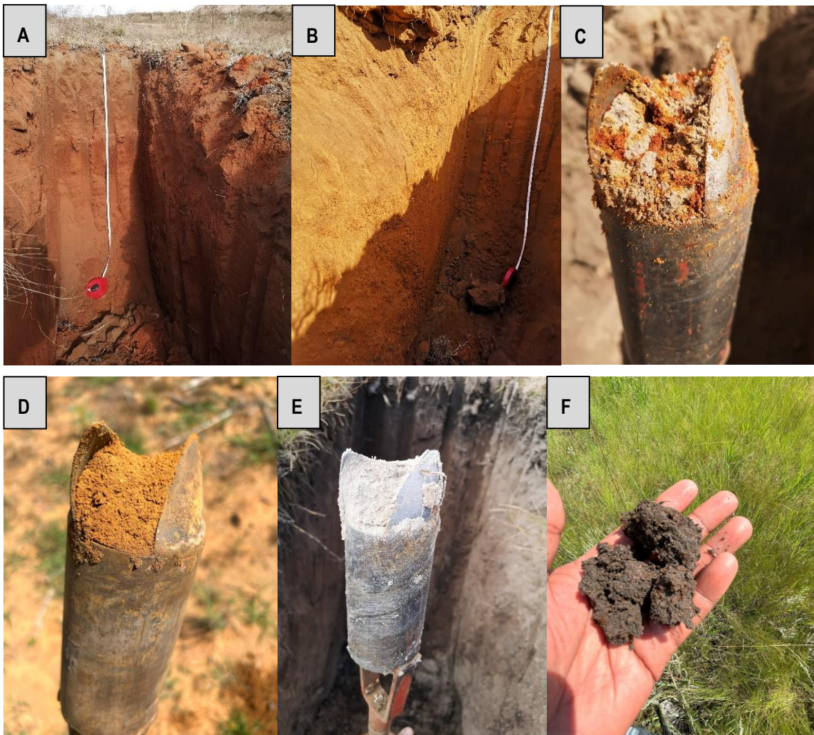
Figure 5-32: Examples of the identified soil forms: A) Hutton (Red apedal), B) Clovelly, C) Longlands, D) Avalon, E & F) Wetland soils (Albic & G)
